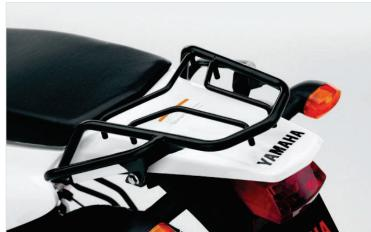
A full accessory lineup of specially developed rear racks is available. Made from strong, durable steel pipe, the flat top makes them practical and easy to strap all kinds of goods down on.
