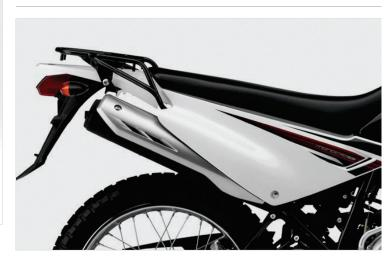
The high-mount exhaust pipe provides plenty of ground clearance and is less susceptible to the effects of exhaust heat. The muffler (silencer) has two expansion chambers and is designed with vents in the chamber partition and pipe length to achieve excellent exhaust efficiency while also producing a gratifying exhaust note.
