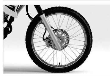
The large-diameter 21-inch front tire contributes to stable handling while the 18-inch rear applies drive force effectively to the surface. Whether riding off the beaten track or on the pavement, you'll get solid performance and excellent wear resistance from these dual-purpose tires.
