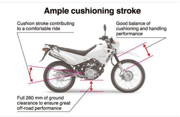
The rear Monocross suspension features a single cushioning unit with the front-end of the shock absorber attached to the frame and the rear end to the rear arm in a way that re-directs the up-down motion of the rear wheel in a slightly diagonal direction to absorb shocks effectively. This rugged suspension layout enables plenty of wheel travel and contributes to great road surface grip and on/off-road performance.
