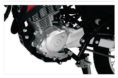
Designed with the latest technology like an optimized clutch dog shape, the transmission's gear ratios are selected with a priority on drivability, good pick-up and agility in around-town riding. Combined with the fuel-efficient engine, the XTZ achieves good mileage characteristics in the practical-use speed range.
